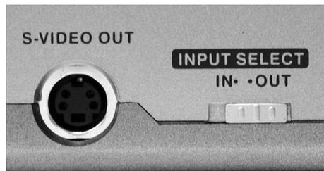
When the **INPUT SELECT** switch is set to **OUT** position, the player is configured to export AV signals to external equipment through its AV input/output jack. When set to **IN**, the player is configured to import AV signals from external equipment.
